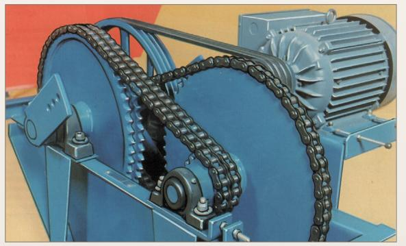
**Drive Unit** uses 10 hp. electric motor. Plunger driven through triple V-belt, double #100 roller chain-and-sprocket drive unit. Large 2-1/2 inch and 1-3/4 inch shafts plus high quality bearings assure durable operation. (Guard removed for viewing).
