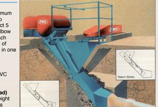
180 (U.S.) gallon hopper can be filled by gutter cleaner or scraper. Constructed of 1/8-inch steel. Approximately 3 ft. by 7 ft. opening at top.
