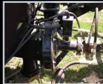
6 Inch Brass Pneumatic Actuated Discharge Valve
