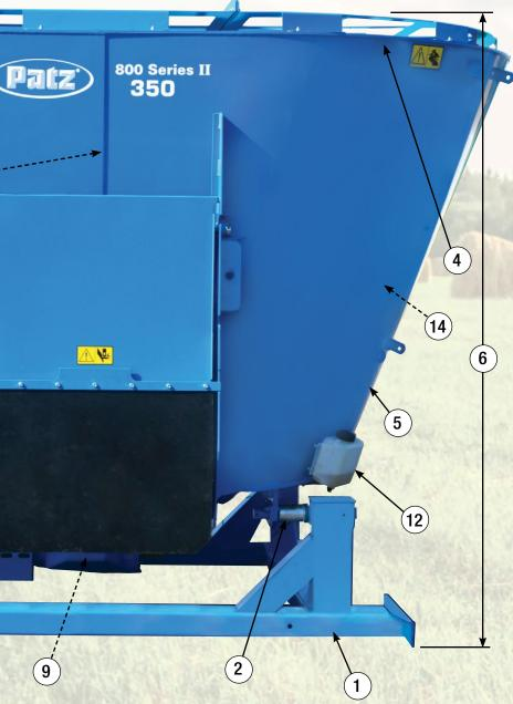
9 **5-year prorated planetary gearbox** warranty. Planetary breather is routed through the bottom plate for easier maintenance and access.
