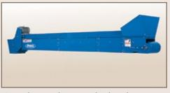
▲ Bolt-together coupler brackets provide reinforcement for extra strength and allow up to 30-foot (9 m) spans between supports. A 100-foot (30 m) conveyor weighs more than 3,100 pounds (1,406 kg) with rugged construction.
