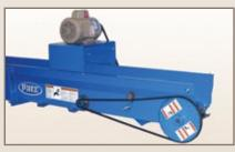
The motor mounts top or bottom for installation versatility. The 162-A uses a single V-belt with roller chain reduction. (Guards removed for viewing.)
