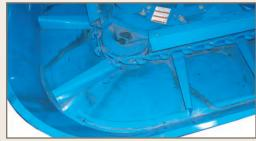
▲ **Corner Sections.** A 90° corner section permits easy turns. A 22-1/2° corner section is also available in double trough sections for added versatility. (Optional chain cover shown above.)
