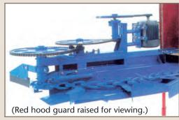
▲ Final-drive roller chain reducer is available with chain speeds of 18 or 30 F.P.M. and with 2 or 3 hp. Economical choice for limited hours of use per day.
