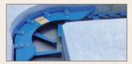
This **Return Corner** is anchored in concrete. A steel wear plate protects the floor. An optional ultra-high-molecular-weight (UHMW) return shoe reduces friction when moving dry material. (Gutter cover removed for viewing.)
