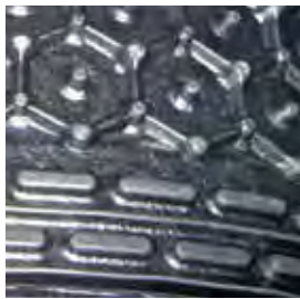
Minimized soiling underneath the mat due to the sealing lips in the rear section
