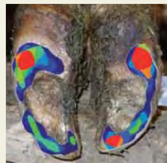
pressure distribution of claws after 6 months exposure to walkways with soft rubber
