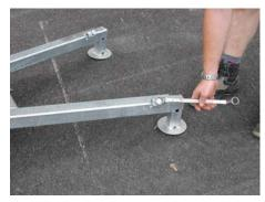
Before you put the mixer into operation, make sure, that the mixer shaft as well as the roller carrier are secured with the corresponding safety pin.
