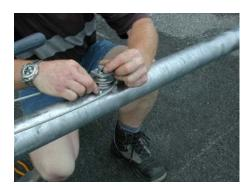
Put the cable starting at the mixer shaft support around the deviating roller ....
