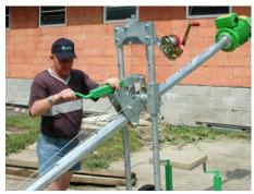
At the same time release the rope with the winch.
