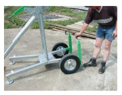
Crank up both supports until the wheels are definitely off the ground. If you have a concrete ground, we recommend to cut in slits for the supports. These supports together with the front support plates absorb the pushing forces occurring during the operation.
