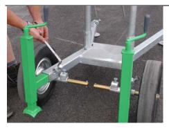
To increase the stability, all four support legs can be adjusted longitudinally.
