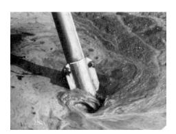
You can go by the fastening clamp of the guard bow. The clamp should still be visible. That way some air gets sucked in at intervals, which enhances the mixing performance without creating a lot of foam.. . When you have slurry with a strong sediment (pig and poultry manure, manure with a lot of sawdust etc.) the mixer shaft should be as low as possible for mixing.
