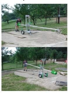
For the transport crank up both supports.
