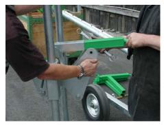
Lock the adjusting spindle in the mixer shaft support.
