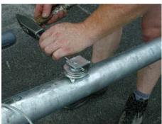
Remove the deviating roller from the mixer shaft....
