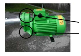
The gearbox of the MEX 450 G is filled with 0,3 I oil type Shell X15W/40. Here, too, the oil only needs to be exchanged in the course of repairs.
