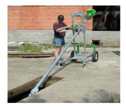
With the rope winch, for lifting and lowering and with the hand lever spindle - for swiveling the mixer shaft - it can be lowered into the pit opening (minimum 60 x 60 cm) without great effort.
