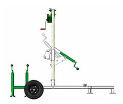
The adjusting spindle can also be mounted turned by 180 °.
