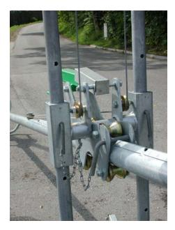
The rollers of the mixer shaft support, the guiding pipe, the bearing of the tires as well as the spindles of the support, have to be lubricated, as required, with a tenacious grease that adheres well.
