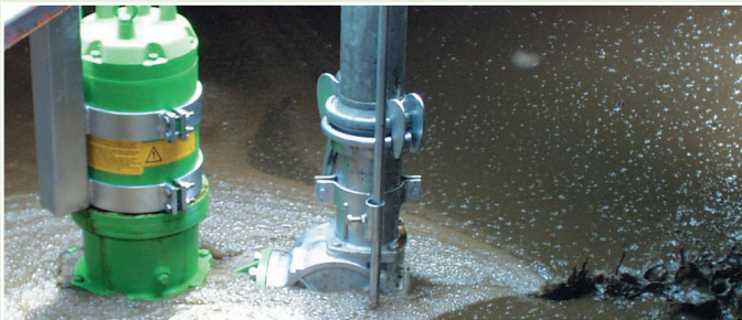
3-way cock with fixed stirring nozzle for 7.5 to 15 HP pump, including rods and delivery connection HK 133 (5 1/4")
