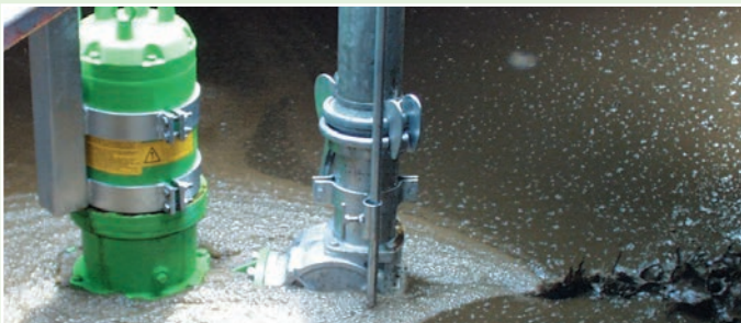
3-way cock with fixed stirring nozzle for 7.5 to 15 kW pump, including rods and delivery connection HK 133
