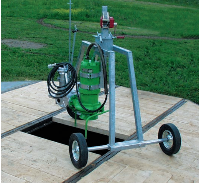
Pump trolley for 3 m immersion depth
